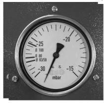
marked in red. The vacuum must be monitored manually. If, for example, a port diameter is 100 mm, and the manometer's needle is on the 100 mark, the filter must be cleaned. This applies correspondingly to exhaust ports of 80 mm and 63 mm diameters. The relationships are shown in the accompanying illustration and the following table.
