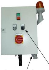
Optionally, the device can be equipped with a start-up through an external potential-free contact. That means a coupling option is established between the suction device and a dust-producing machine connected to it. In this way, the dust-producing machine starts and stops the suction device automatically. The toggle switch on the switch box must be set to "AUTO" for this operating mode. As previously described, the suction device is operated in the "MANUAL" position.
