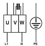
To connect the cables, remove the outlet element. Open the required cable entry openings on the terminal box. Carry out the connection as well as the layout of the jumpers according to **1 circuit diagram**. Connect the protective conductor to the terminal with the following symbol: ①.
