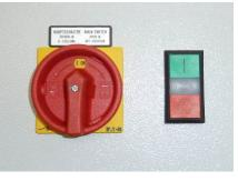
down, always switch the system off from the OFF switch first, wait for the postcleaning to complete and then activate the main switch.
